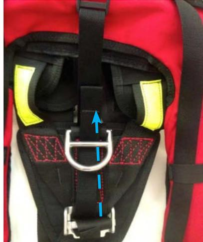
2) Route bottom end of collar back attachment strap up between adjuster center bar and upper D ring webbing. Continue through webbing slot of D ring.
