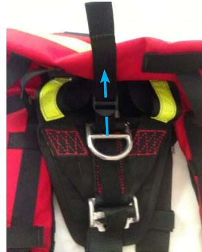
3) Continue up through inner slot of back attachment adjuster and then down through the outer slot to lock webbing. Reinstall Velcro keeper in back attachment strap end.
