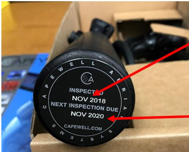
When you receive the SEA LV2, the laser etched “INSPECTED” date is the date that Capewell completed a factory inspection prior to shipping the product.
